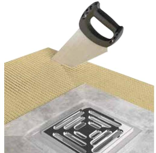
Your **DeltaTray** can be trimmed enabling the tray to be altered slightly to suit installation tolerances and also to overcome issues that may arise if the drain position becomes obstructed by joists under the floor. Trimming the tray will reduce the thickness of the tray on the sides that are to be trimmed. It is very important that after trimming, the cut sides of the tray are not reduced by more than 2mm of the original tray thickness.
